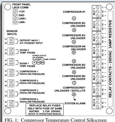
If the Control fails or in suction high/low alarm, all control relays are de-energized, the Switchback relay is energized and power is switched to the backups. The mechanical backup controls now operate the compressors based upon their Cut-IN and Cut-Out settings. With this method, the backup settings can be set to run the rack as close to the temperature set point as possible.
