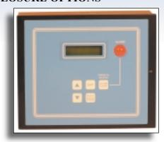
**NEMA 1 Compliant Enclosure** - This enclosure is intended for indoor use only primarily to provide a degree of protection against contact with the enclosed equipment. The enclosure is not designed to provide protection from water or to be placed in a hazardous environment. Mount only in Pollution Level 2 environments, i.e.. Environmentally controlled offices, control rooms, or environmentally controlled machine rooms.
