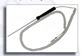
**FOOD PROBE WITH COIL CORD** - The Temperature Sensor is a high-precision NTC thermister. The sensor probe is a 6 inch long stainless steel thermistor with a 5 second reaction time rating. The coating is highly resistant to most solvents and chemicals. It is connected to a 30 foot coil cord.
