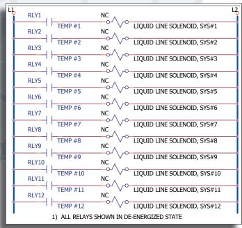
Alarm Monitoring Mode - Zone Specific Alarm Relays -- (SPDT) These relays are assigned to indicate a High or Low Temperature Alarm Condition for their assigned tempeature sensor. These relays can be configured to Energize to Open or Energize to Close.
