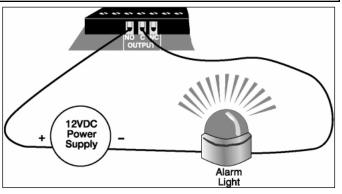
**NOTE:** For safety reasons it is highly recommended that the unit only be used to switch low voltage signals (30 volts or less). If you intend to control higher voltages you must install the unit in an NEC approved electrical panel or enclosure and have wiring performed by a qualified electrician.
